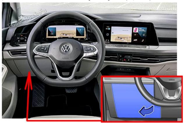
Right-hand drive vehicle: Push the damper element up and into the opening in the bracket, before pulling it out side-ways (1). Push the catches up in the direction of the arrow while at the same time opening the storage compartment further (2).
